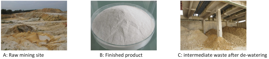
Fig. 1. Mining and further processing of kaolinitic clay
