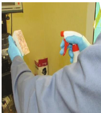
Fig. 5. Application of the phe-nolphthalein
