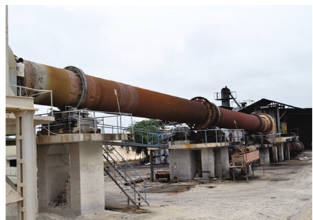
Fig. 2. Calcination in rotary kil
