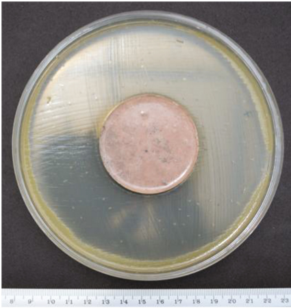
Fig. 5. Activity evaluation against S. aureus of a geopolymer cement disk with 0.5% (w/w) of Triclosán. A 116 mm Halo was developed on it.
