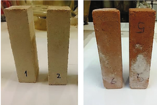
Fig. 3. The specimens after dried at constant ambient temperature: (ED)M on the left; (FC)M on the right.
