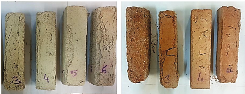
Fig. 4. (ED)M after 20 freeze-thaw cycles (on the left); (FC)M after 9 freeze-thaw cycles (on the right).
