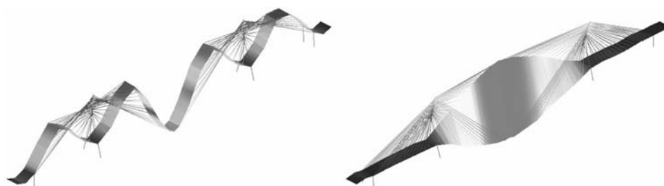
Figure 3. Guediana Bridge mode shapes extracted from Multi-run ambient vibration data.
