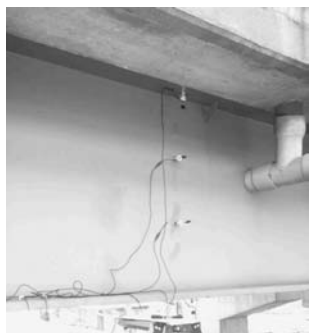
Figure 3. Search of neutral axis by Strain Checker.
