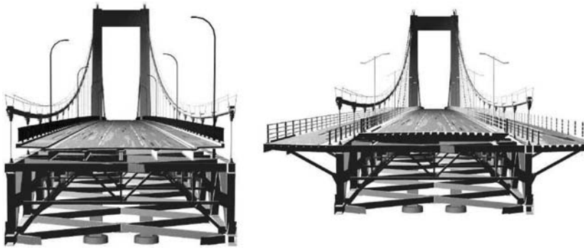
Figure 2. Bridge section at midspan before and after strengthening and widening.
