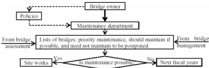
Figure 4. Procedure of bridge maintenance.
