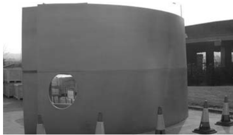
Figure 6. The 1:1 mock-up of the stainless steel shell.
