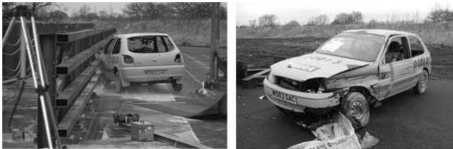
Figure 15. Parapet impact test for 4-rail type parapet.
