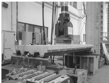
Figure 2. Static flexural test set-up.
