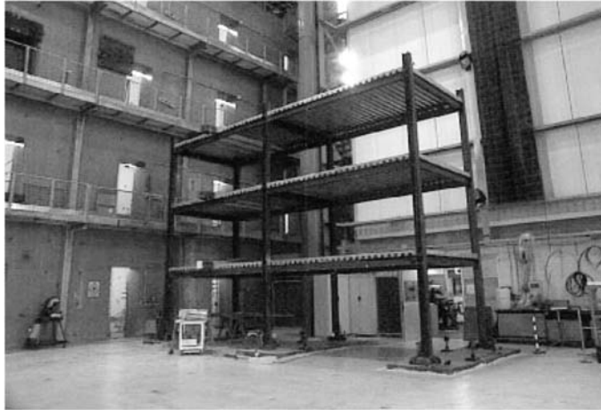
Figure 1. The “Baby-Frame” specimen at the ELSA laboratory of the JRC in Ispra, Italy.
