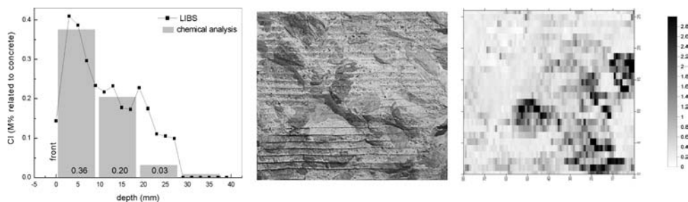
Figure 1. Left: Comparison of chlorine depth profiles measured on a concrete core originating from a marine structure by LIBS and chemical analysis results. Right: Photograph of measured surface (crack layer) and chlorine distribution. Cl-contents in M%/cement.
