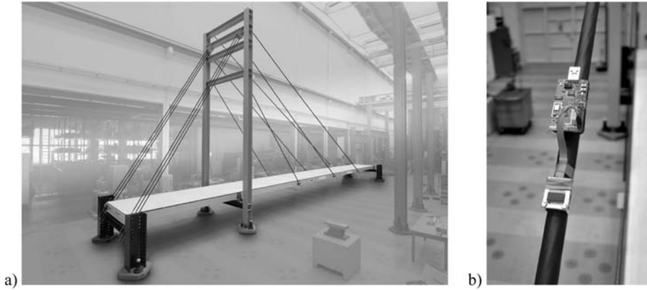
Figure 1. a) Laboratory stay cable bridge. b) Network node mounted on a cable with transceiver (top) and accelerometer (bottom).
