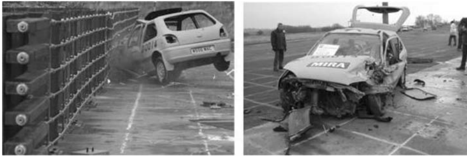
Figure 14. Parapet impact test for tension wire parapet.
