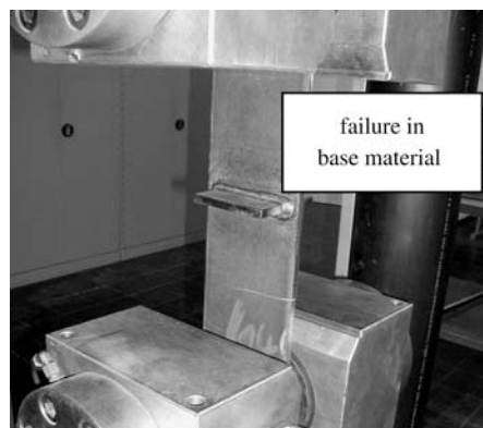
Figure 2. Fatigue failure in the base metal.
