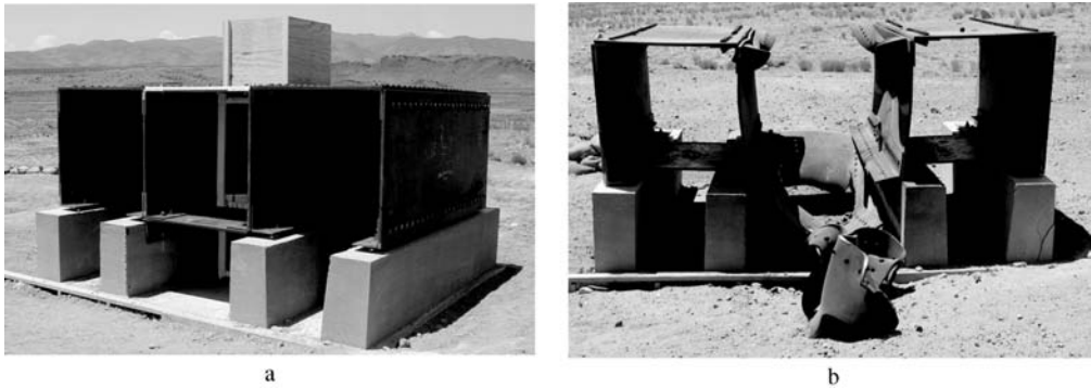
Figure 3. Steel cellular tower section, pre-test (a) and post-test (b).
