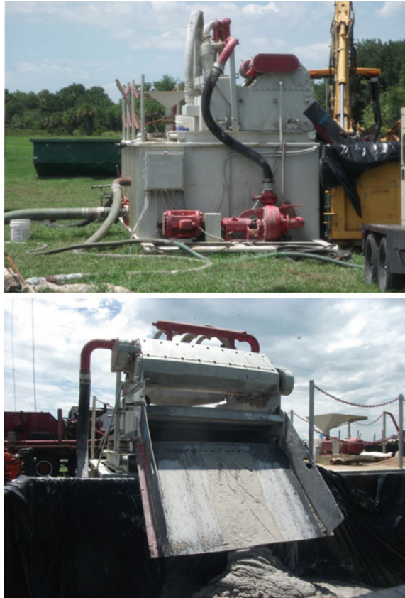
Fig. 6.6 Desanders and shale shaker used to separate cuttings from the drilling mud
