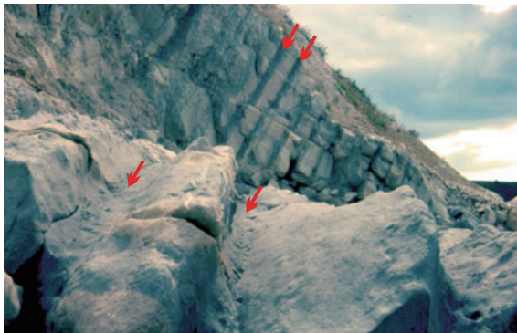
Fig. 4.11 Lower chalk (Dorset, England) with a well-developed alternation of relatively pure white chalk beds and grayish clay-rich marl beds (arrows)
