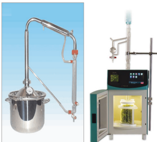
Fig. 1.2 Conventional and innovative (microwave) Clevenger for extraction of essential oils
