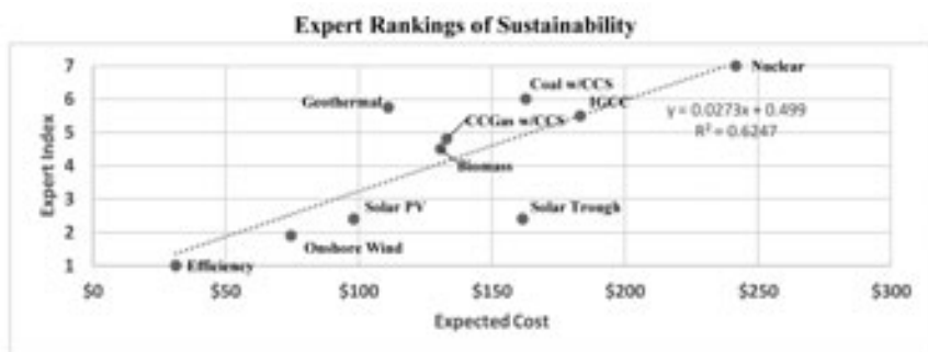
Figure 11.6 Multicriteria Portfolio Analysis Compared to Qualitative Ratings Sources: Shimon Awerbuch and Spencer Yang, "Using Portfolio Theory to Value Power Generation Investments," in Analytic Methods for Energy Diversity and Security , ed. Morgan Bazilian and Fabien Rocques (Oxford, U.K.: Elsevier, 2008), 63, citing International Energy Agency/Nuclear Energy Agency, Projected Costs of Generating Electricity (Paris: OECD, 2005); Ron Binz, et al., Practicing Risk-Aware Electricity Regulation: What Every State Regulator Needs to Know (Boston, MA: Ceres, 2012).
