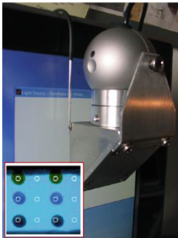
Fig. 22.7 Arrangement of a CSPT-based electronic nose. The screen is the light source used to probe the sensing layer that is imaged by a webcam. In the inset the imaged sensing layer. Circles indicate the region of interest whose pixels intensities are averaged and considered as the sensor array response
