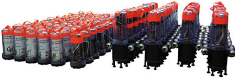
Fig. 23.16 The two main types of floating sensors. On the left , the passive sensors that are driven by the flow. On the right , the sensors that have a propeller to maneuver them when encountering obstacles. Reproduced with permission from reference (85)
