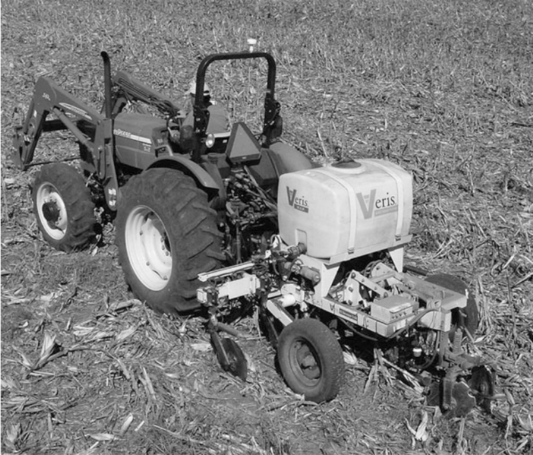
Fig. 2.6 Commercial sensor system integrating soil electrical conductivity and pH mapping (Veris pH manager, Veris Technologies, Salina, Kansas, USA)
