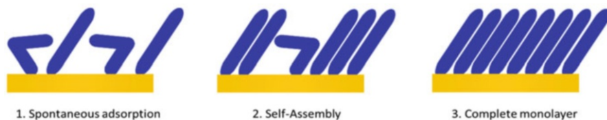
Fig. 16.7 Schematic representation of the two-step process leading to the formation of a complete monolayer
