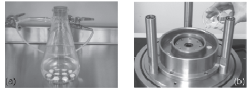
Figure 2. Saturation of HAEV ceramics: (a) vacuum beaker, (b) in-place water bath.
