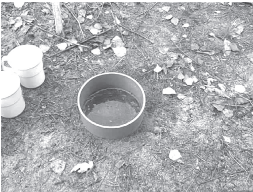
Figure 1. Beerkam infiltration test at null pressure head.
