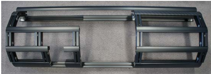
Figure 4: Skeleton structure assembled and lacquered.
