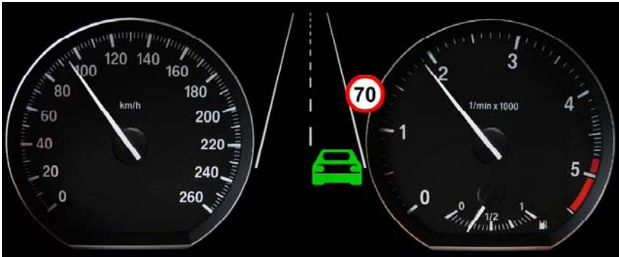
Figure 1 Anticipatory assistance system during an approach of a speed limit advice with coasting advice (green ego car)
