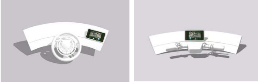
Figure 5 Touchscreen location on the dashboard in two proposed versions of a steering device.
