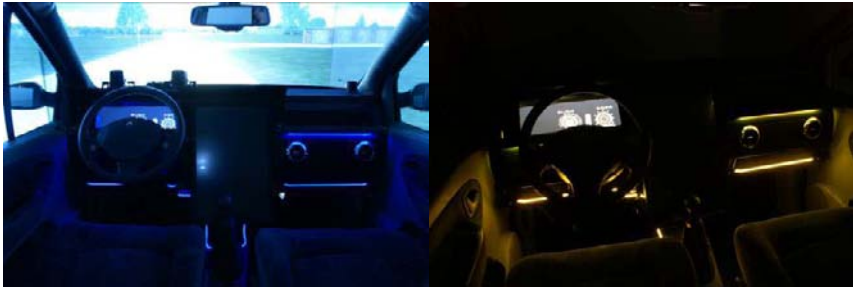
Figure 9: Ambient in car lighting and display lighting of the Fraunhofer IAO driving simulator at different light conditions.
