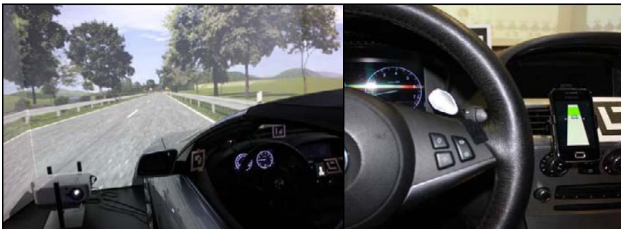
Figure 1: (left) static driving simulator with BMW mockup, (right) mobile phone mounted beside the steering wheel
