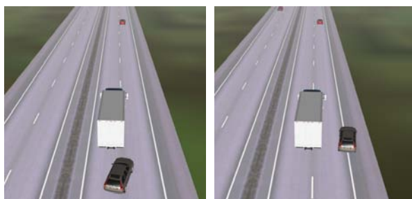
Figure 5 The LCDA scenario with host vehicle (truck) entering back into right lane, and hidden vehicle suddenly appears from behind into subject's right side blind spot.
