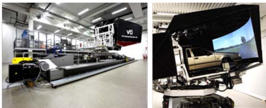
Figure 1 The VTI driving simulator III with the moving base platform and a car cabin mounted on it.
