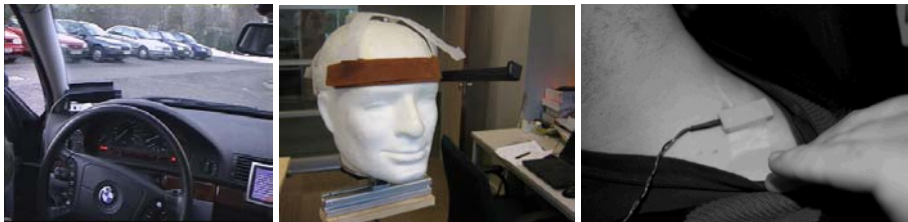
Figure 4 shows different stimuli: 1) visual stimuli as LED in the cluster instrument 2) a visual stimulus fixed on the head 3) A small vibrator mounted on the shoulder of the test subject
