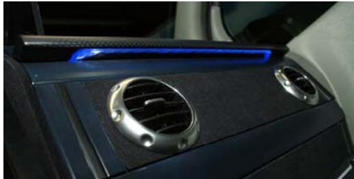
Figure 7: Installation of ambient light.
