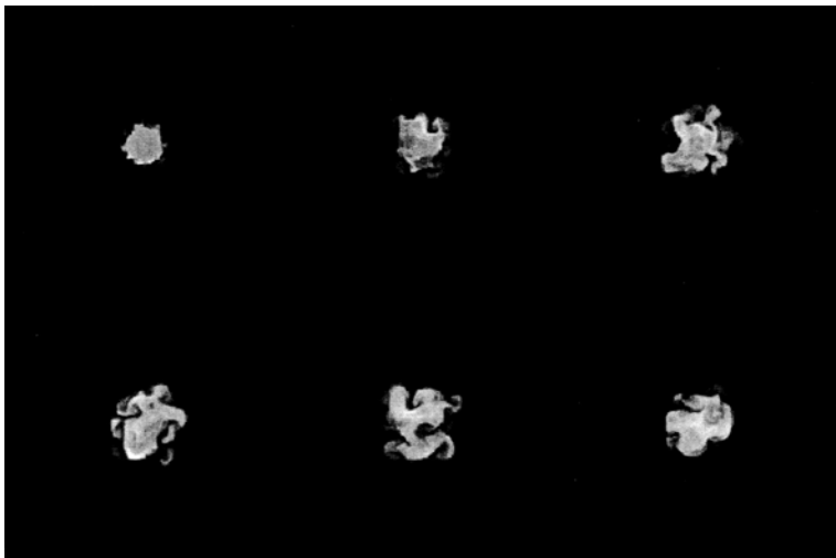
Fig. 15.20: Gray-scale temperature plots of cross-sections through a three-dimensional hydrodynamic jet that becomes increasingly unstable along its length. (Lighter gray indicates higher temperature.) Cuts are taken along the jet length at (7.5, 15.0, ..., 37.5, and 45.0) jet radii. While jet is roughly laminar early on, it becomes more turbulent downstream. Reproduced from Fig. 10 of [556], by permission of the AAS.
