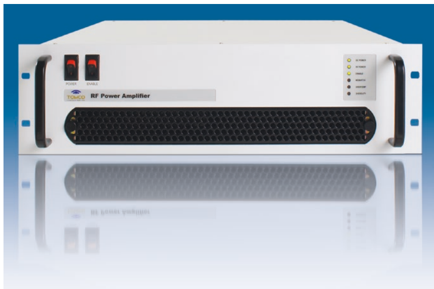
Fig. 4.7 A TOMCO BT-AlphaS Series RF Amplifier suitable for PFG NMR applications. This amplifier operates from 100 kHz to 30 MHz and has a nominal output power of 500 W. Important status parameters such as load mismatch and amplifier temperature status are available via a digital interface (photo courtesy of TOMCO Technologies)
