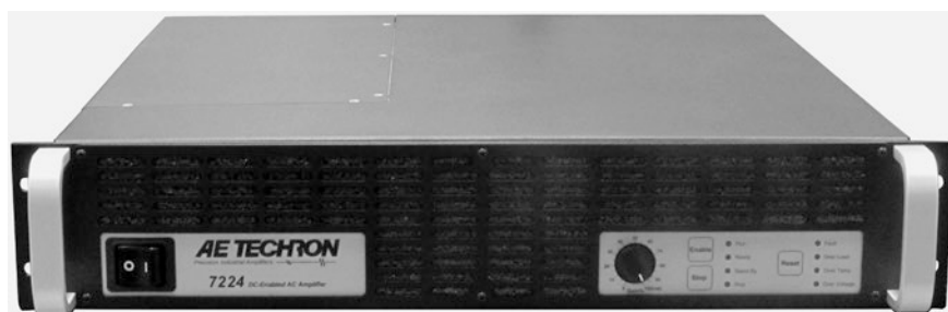
Fig. 4.4 A 7224 AE Techron NMR/MRI Gradient Amplifier, a linear amplifier capable of performing PFG NMR experiments on low field permanent magnet based systems (courtesy of AE Techron Inc)
