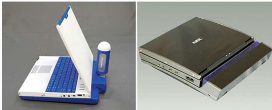
Fig. 9.11 NEC's laptops powered with DMFC. Left : DMFC coupled to the refilling tank (2003), right : second generation (2004) (Reproduced from Ref. [58] with permission)
