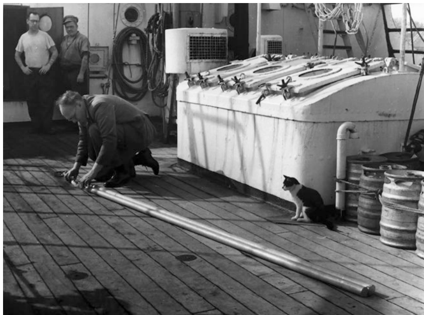
Fig. 4.2 The first neutrally buoyant float for tracking water movements at depth was developed by John Swallow, a British oceanographer. It consisted of an aluminium pipe with a battery and timer circuit that would excite a magnetostrictive transducer, a “pinger”, hanging underneath. John Swallow pictured, 1955. (Image from the Archives of the National Oceanographic Library, National Oceanography Centre, Southampton.)
