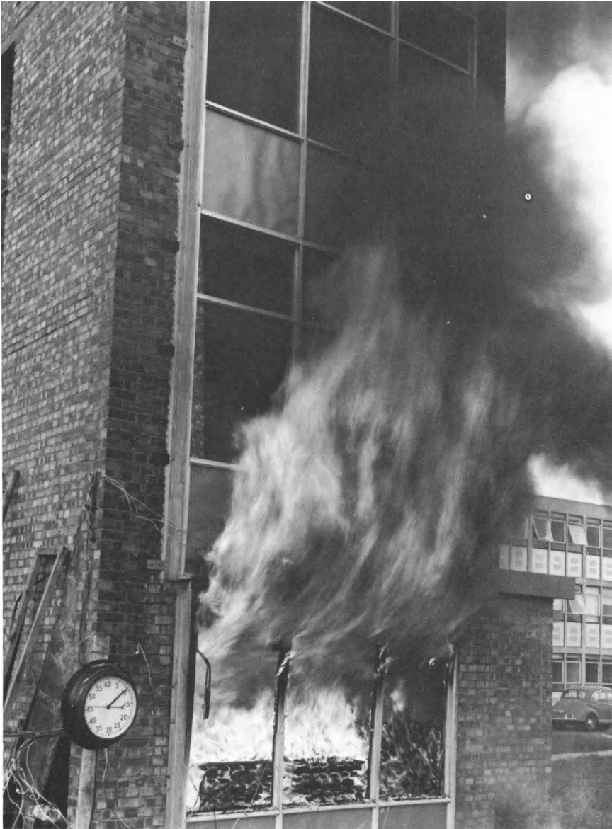
Figure 7.10 'Full scale' fire test on GRP cladding panels. Note: the controlled fire load burning at ground level, the time from ignition (10 minutes) and the unignited curtain fabric in the first floor window. Such full scale fire tests, despite the limited extent of building involved, are quite rare
