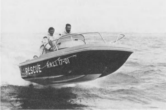
Figure 1.1 17 ft high-speed rescue boat. Moulded in GRP sandwich construction
