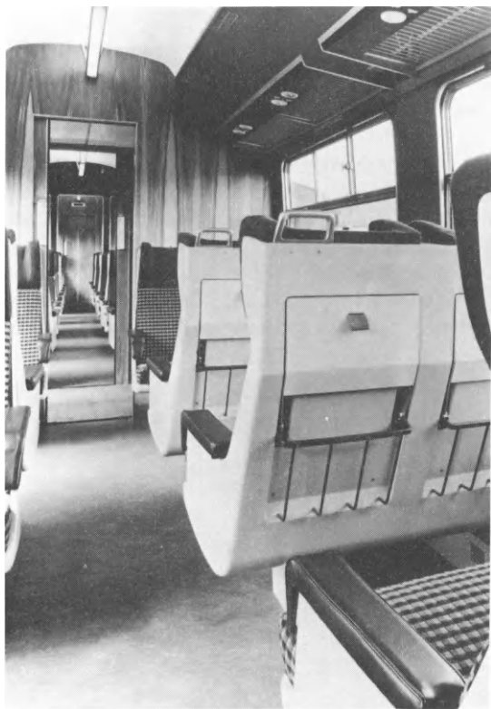
Figure 2.4 Train seats cold press moulded in GRP
