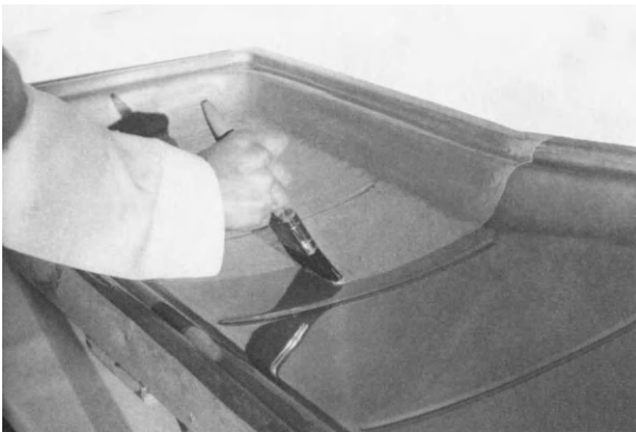
Figure 5.2 Brushing on gel-coat
