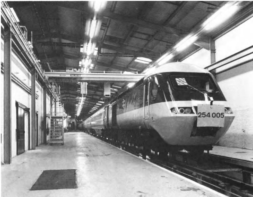
Figure 2.3 British Rail high-speed train with driver's cab made from impact resistant GRP foam sandwich
