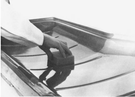
Figure 5.1 Applying release agent to the mould
