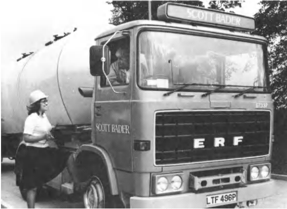
Figure 2.2 A truck cab with GRP panels
