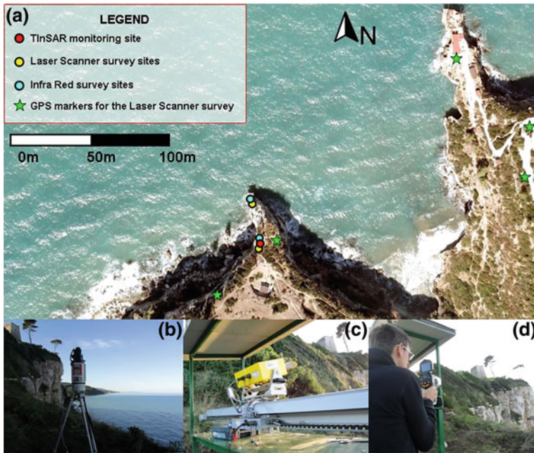
Fig. 3 Plan view of the sensing sites and GPS stations. a Photos of the instruments’ installations: Riegl VZ400 laser scanner; b IDS IBIS-L GBSAR; c NEC TH7700 thermocamera; d All subfigures have been modified from Martino and Mazzanti (2014)
