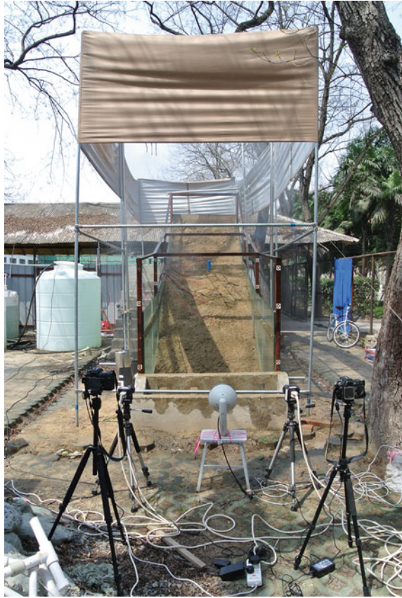
Fig. 2 The stereo-camera systems implemented in front of the scaled-down slope of the landslide simulation platform
