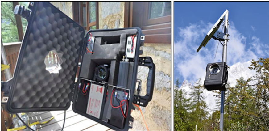
Fig. 1 Left the watertight IP67 box housing the system. Right one of the system units and the solar panel installed on a pole
