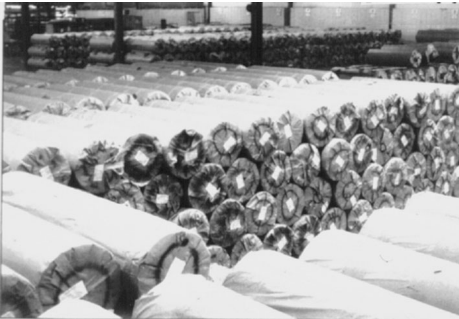
Figure 4-11. Rolls of Calendered Geomembrane Being Stored before Fabrication into Panels.
