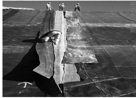
(b) Separation of GCL panels \approx 200 mm (8 in.)
