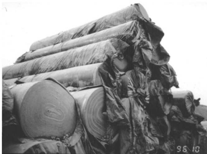
Figure 7-7. Thick Needle-Punched Nonwoven Geotextiles Used as Protection.
