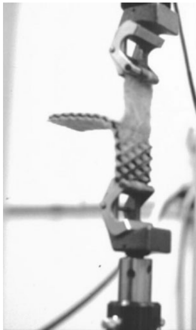
Figure 7-12. Ply Adhesion Test of a Geotextile Thermally Bonded to a Geonet Core.
