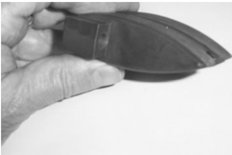
Figure 4-19. Photographs of Wedge Welding Devices, Details of the Device, a Dual-Track Wedge, and a Cross Section of the Subsequent Seam.
