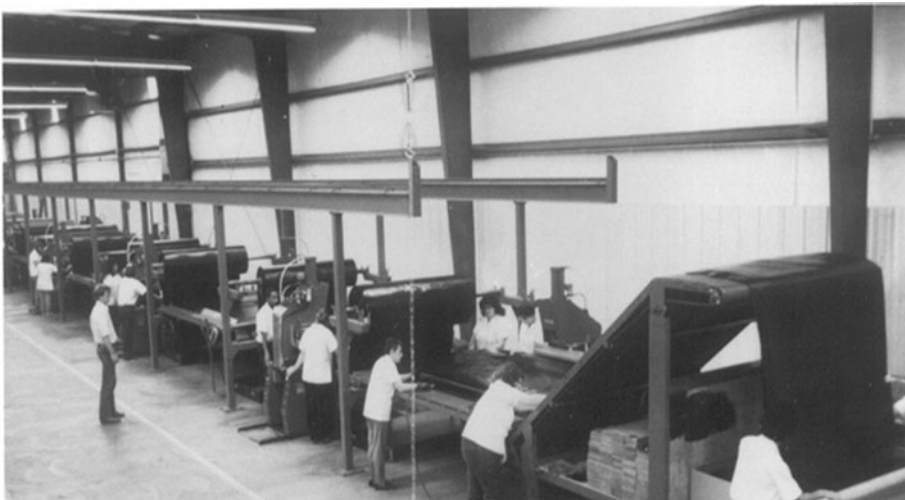
Figure 4-13. Factory Fabrication of Calendered Rolls into Accordion-Folded Large Panels for Field Deployment.
