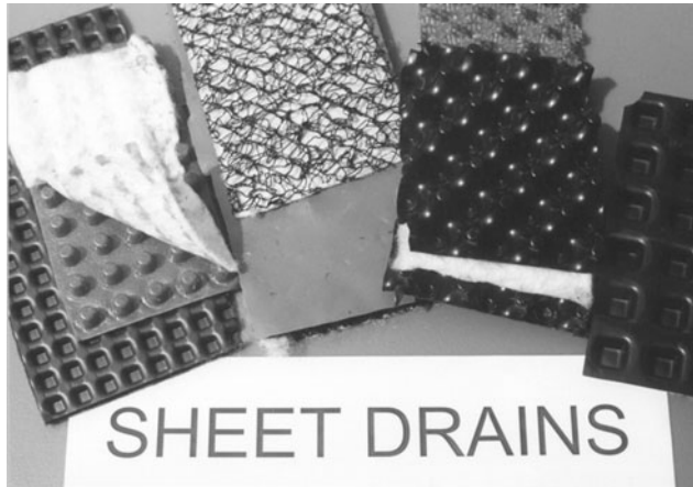
(a) Geocomposite sheet drains
