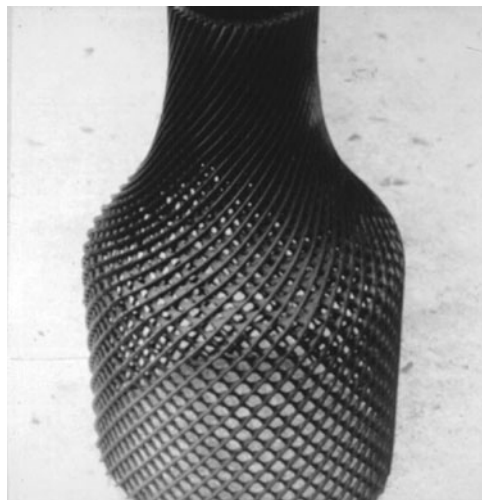
Figure 7-9. Counterrotating Die Technique (top sketch) for Manufacturing Biplanar Drainage Geonets and Example of Laboratory Prototype (bottom photo).
