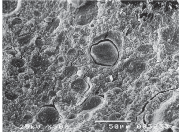
Fig. 6.57 Irregular domains of compact C–S–H gel in the paste after 1,200 days of curing in the chloride solution. (According to [246])
