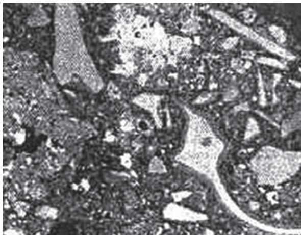
Fig. 1.4 Microstructure of light concrete from El Tajin under SEM
