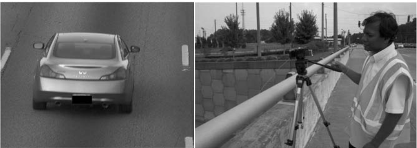
Figure 1: HD Camera Set-up and View
