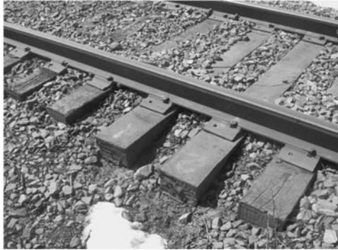
Figure 2: Plastic test ties showing no signs of degradation while rail spikes hold steady.
