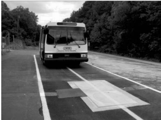
Figure 2 – Bus Entering Wireless Charging Area
