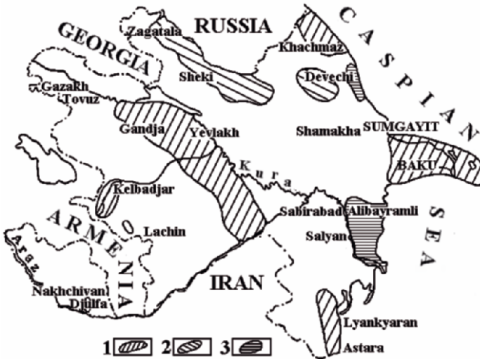
Figure 2. A schematic map of zones in the Republic of Azerbaijan where thermal waters might be utilized: 1. Prospective zones for exploration for thermal waters. 2. Local, unexplored areas. 3. Non-prospective zones.
