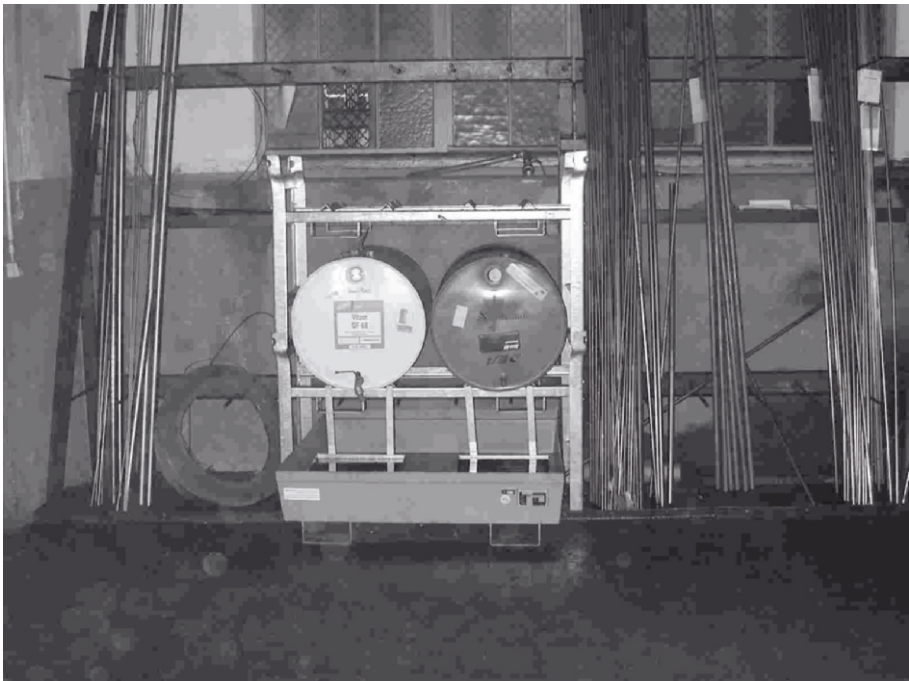
Figure 4. Retention tray with the possibility to secure barrels and safely transport them by a fork-lift.
