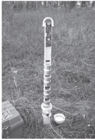
Figure 4. Rail with sensors being inserted into the access tube.
