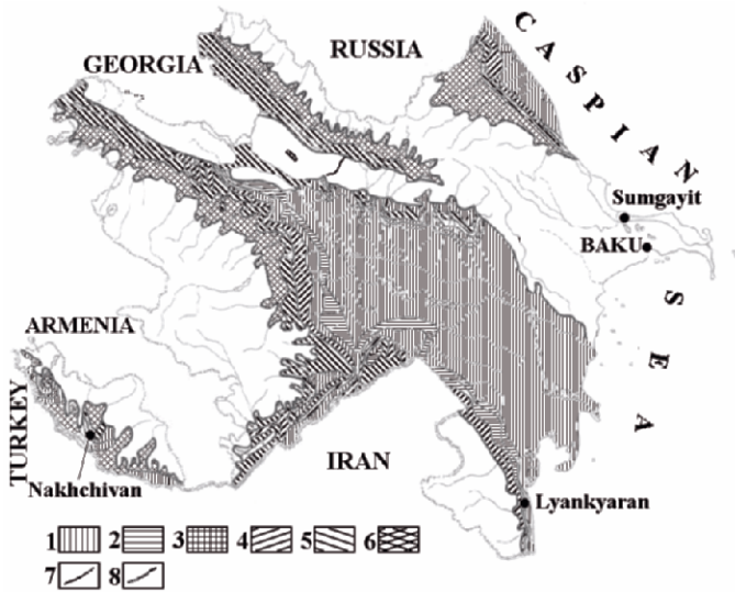
Figure 3. Lithological composition of aquifers in continental deposits of low-lying regions, Azerbaijan. Variations in gravel content of the water-containing rocks is as follows: 1 = practically absent; 2 = up to 25 %; 3 = 25-50%; 4 = 50-75%; 5 = 75-90%; 6 = 90-100%. Boundary keys as follows: 6 = areas with different shingle content in the section; 7 = alluvial-proluvial and lowland plains).
