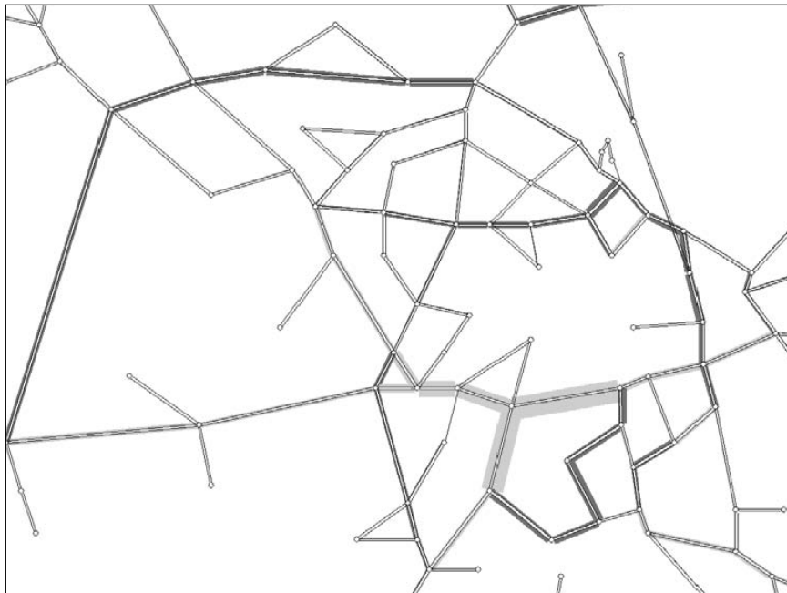
Figure 18.13 Difference between equilibrium solution and side-constrained equilibrium solution satisfying the management goals
