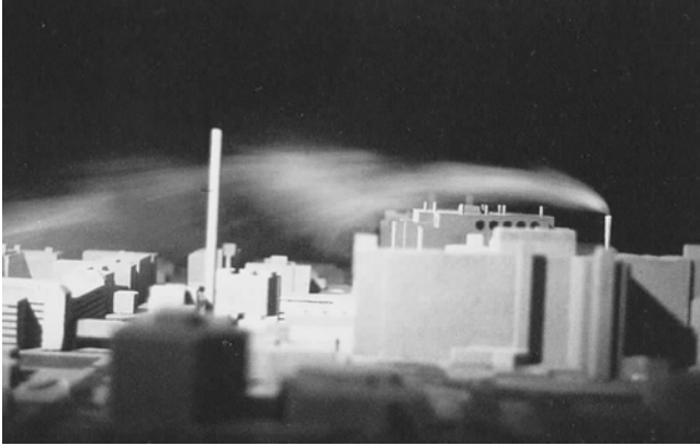
Figure 29. Flow visualization of exhaust plume from a hospital stack (Courtesy of Cermak Peterka Petersen (CPP) Inc.).
