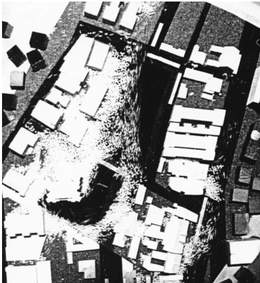
Figure 33. Urban flow visualization with foam plastic beads (Courtesy of Richard Aynsley).
