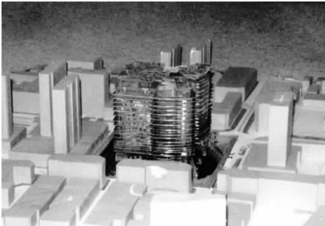
Figure 24. Model of the National Library, Singapore model in a boundary layer wind tunnel (Courtesy of Richard Aynsley).
