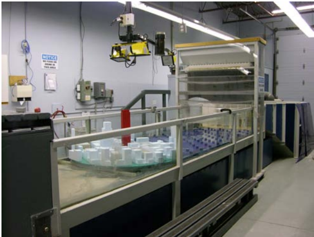
Figure 21. Water tunnel for snow drift modeling at RWDI (Courtesy of Rowan Williams Davies and Irwin Inc. Guelph, ON Canada).
