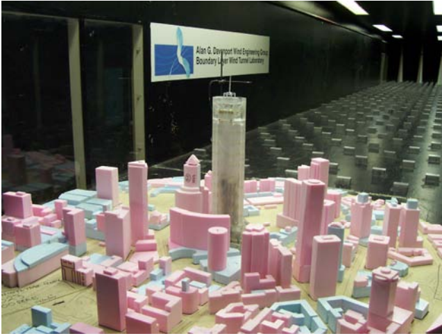
Figure 35. An Urban Model inside a Boundary Layer Wind Tunnel (Courtesy of Boundary Layer Wind tunnel Laboratory, University of Western Ontario).
