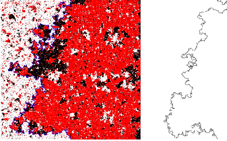
Fig. 3.7 On the left , example of an interface between two clusters of different spin states in the 3-state Potts model with fluctuating boundary conditions. Each pixel is a spin and its colour (black, white or red) corresponds to one of the three possible states. The interface is plotted in blue. On the right , only the interface is plotted
