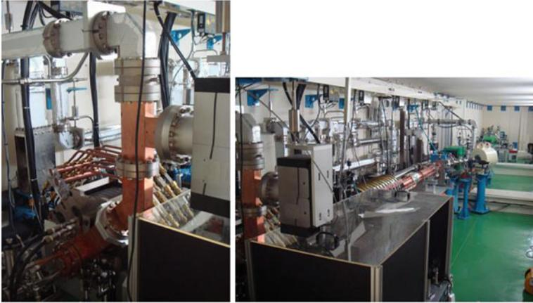
**Fig. 8** Photocathode RF-gun and the accelerating column
