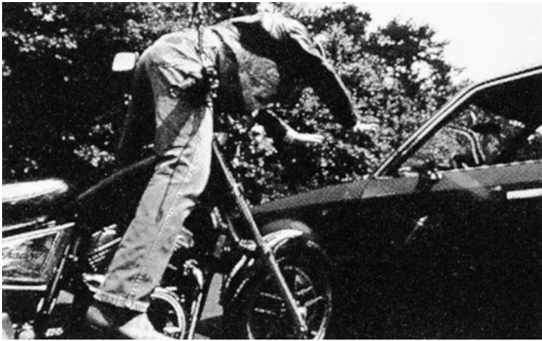
FIGURE 15.16. In a bicycle impact, the bike stops its forward motion, and, on impact, the occupant continues forward, impacting the legs into the handlebar or ejecting the occupant completely from the vehicle. (Reprinted with permission of Elsevier from McSwain et al. 9 )
