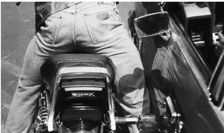
FIGURE 15.17. Off-center impacts tend to center the motorcycle into the vehicle, and the leg is trapped between the two, producing injuries. (Reprinted with permission of Elsevier from McSwain et al. 9 )
