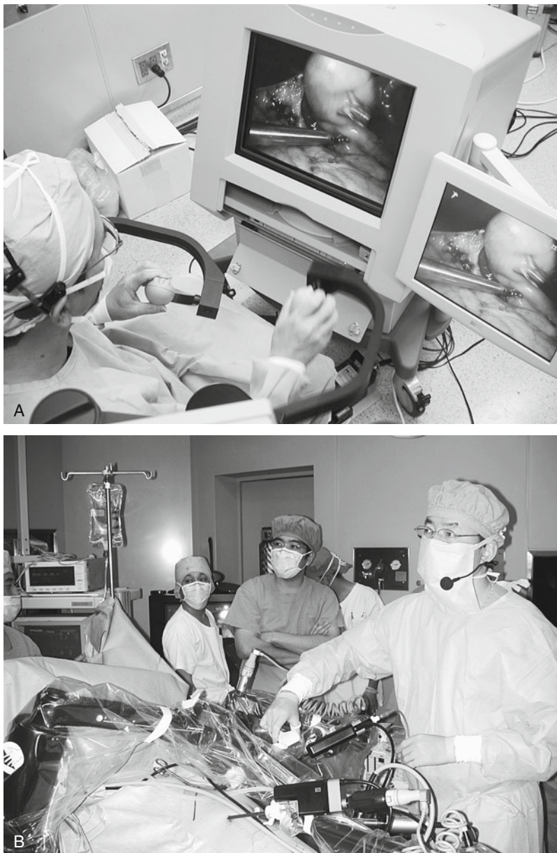
FIGURE 51.9. The ZEUS robotics system. A cholecystectomy was carried out in a teleconference including the European Institute of Telesurgery, University of Strasbourg, France, and the operating theater of Osaka Medical College, Japan. (A) The operator and a manipulator (a master robot). (B) The patient and robotics arms (a slave robot).
