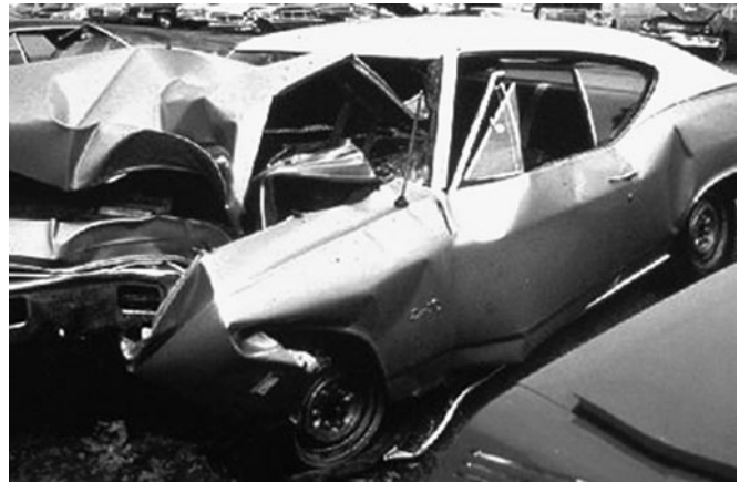
FIGURE 15.2. The energy of the collision is absorbed at the point of impact, but the rest of the vehicle continues to move forward until the remaining energy is absorbed by the ending of the metal in other parts of the car.
