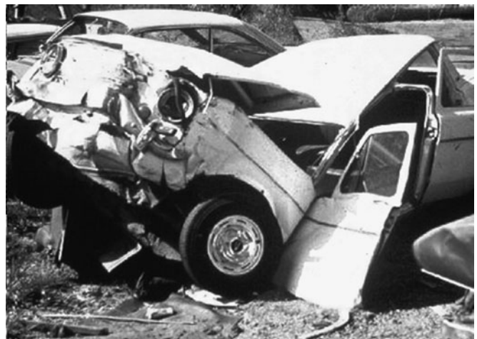
FIGURE 15.3. The entire front of the car is involved in the impact, but the energy of the continued motion of the rear of the car is not absorbed until the body parts bend.
