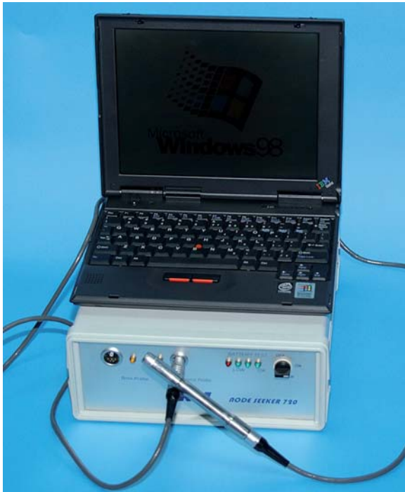
Fig. 8.10. The gamma probe used for intraoperative localization of parathyroid glands in patients with biochemically proven hyperparathyroidism
