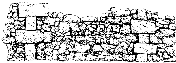
2. Walls constructed of fieldstones and dressed stones, Megiddo. Megiddo I, p. 11, Fig. 13.
