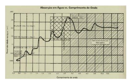
**Fig. 71.1.** The wavelength of light emitted by an erbium–YAG laser is 3 times smaller than that of a CO<sub>2</sub> laser and its absorption in water is 10 times larger than that of the CO<sub>2</sub> laser. This means that erbium laser radiation is absorbed more by the blood, does not coagulate the blood vessels and does not produce thermal damage in the deepest dermal layers
