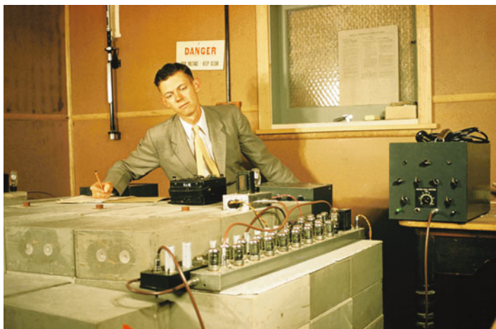
Fig. 6.3-1 An eight-counter IGY neutron monitor established in a small hut at an altitude of 725 m on the slopes of Mt. Wellington, Tasmania, in 1956. Note the large number of “vacuum tubes” that were needed to perform the simplest of tasks prior to the advent of solid-state electronics and the digital computer. The student checking the instrument is one of the authors of this book (collection McCracken)
