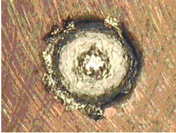
Fig. 7 Impact on the wheel (optical)
