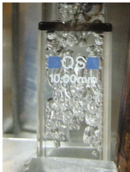
Fig. 9 Inhomogeneous PDMS/KOH after irradiation
