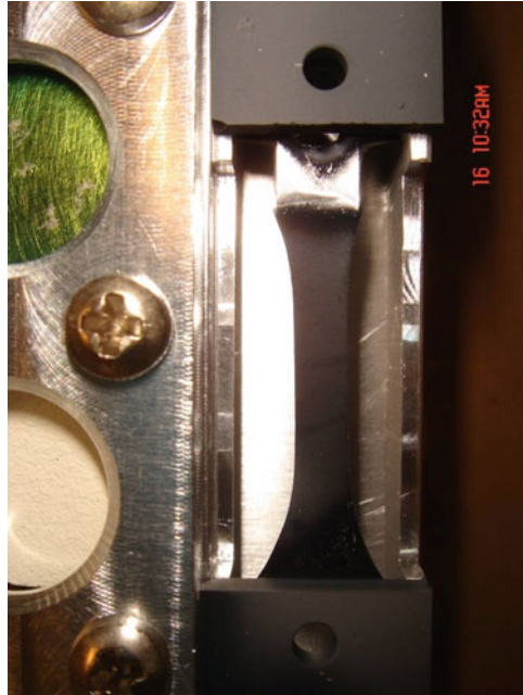
Fig. 2 Kapton XC flown on ram side of MISSE 6 (AO-S-1) showing stretching of the sample at the silver area at the top of the sample in the photograph
