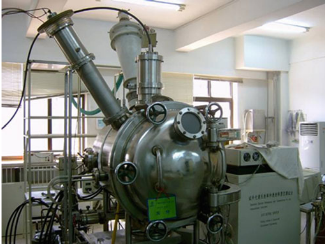
Fig. 4 Combined environment test facility
