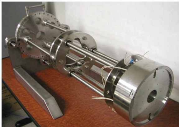
Fig. 4 Sample holder/sample transfer system (front view). The thermal control platform disks (not shown) are attached to the front of the holder
