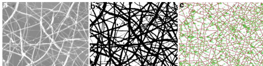
Fig. 1 Optical micrograph of silicone DC93-500 exposed to 8.43 E21 fluence atomic oxygen in lower Erath orbit during MISSE 2 mission. (a) Original picture. (b) Convert original picture into black crack and white non-crack area. (c) Convert all cracks into thin lines
