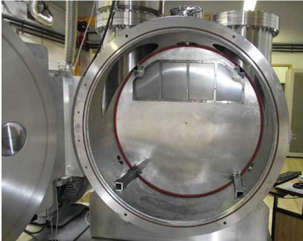
Fig. 3 Dust filter installed in the simulator chamber
