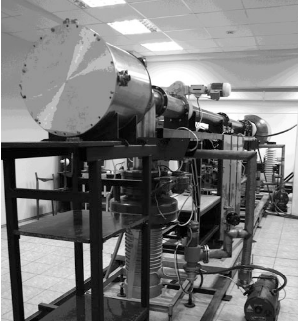
Fig. 1 The linear accelerator for simulation of micrometeoroid impacts
