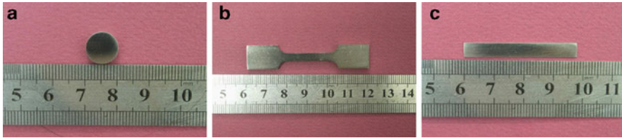
Fig. 1 Typical Nano-Indentation test and XRD specimen (a), tensile test specimen (b) and DMA specimen (c) used in this study
