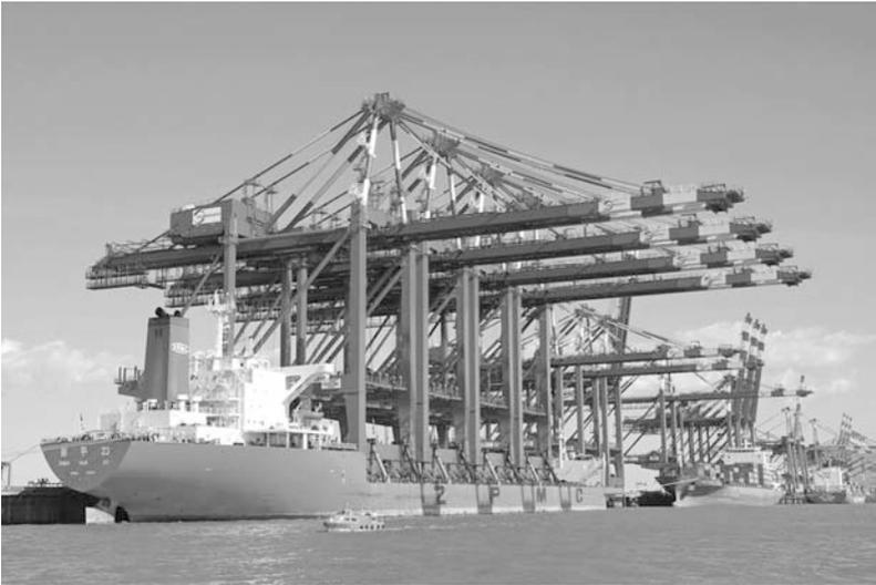
**Figure 1.1** ZPMC transport vessel with assembled cranes
