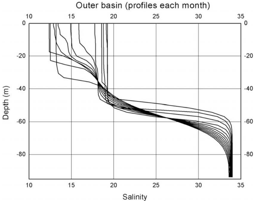
Fig. 5.2 The salinity response in the outer basin over a one-year run
