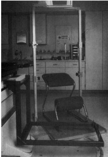
Fig. 31.13. A special couch extension designed to reproduce the standing TBI treatment position when treating the electron chest wall boost fields. The device is separated into two pieces for ease of handling and, since it is attached directly to the couch, it has the same range of motion as the couch. Patients up to approximately 5 feet tall can be treated in the standing position, while taller patients are treated in a seated position. This style of chair keeps the back of the patient in about the same orientation when seated as when they are standing
