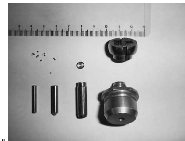
Fig. 11.7 a Disassembled and b assembled Gamma Knife source in bushing
