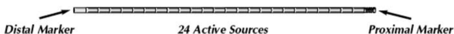
Fig. 33.3. Strontium-90 seeds of 2.5 mm length (60-mm long source train) and radio opaque markers at both ends for radiographic visualization
