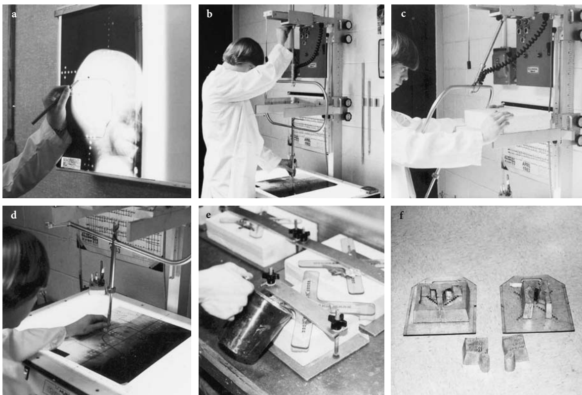
Fig. 5.27a–f. Composite photographs illustrate the low melting alloy shielding block design and fabrication process. a Physician defining the treatment volume on the X-ray simulator radiograph. b Physics technician adjusting the source-skin distance and skin-film distance of a hot-wire cutter to emulate simulator geometry. c Proper-thickness foam block aligned to the central axis of the cutter. d Foam mold cut with hot-wire cutter. e Foam pieces aligned and held in place using a special clamping device. Molten alloy is poured into the mold and allowed to harden. f Examples of typical shielding blocks cast using this system. (From PURDY 1983)
