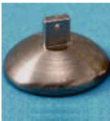
Fig. 8.13. Photograph of protective eye shield composed of lead with a gold covering
