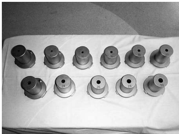
Fig. 11.9a,b. Linac collimators a in place and b various sizes
