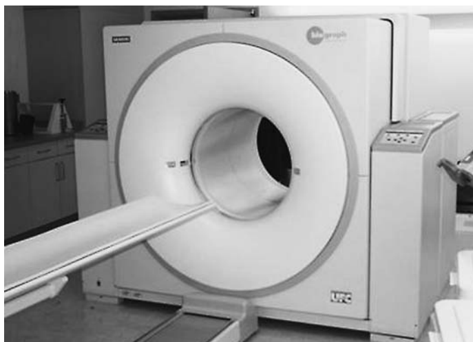
Fig. 6.11 A combined PET/CT scanner
