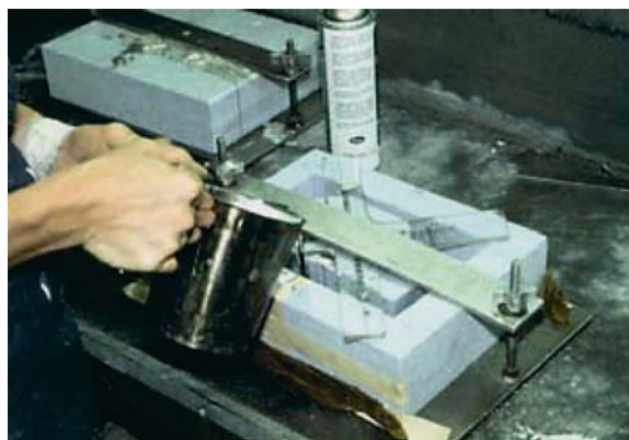
Fig. 8.9. Photograph displaying molten alloy being poured into the form of shaped foam for purposes of casting a shaped field block
