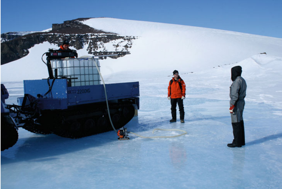
Fig. 6.3 Supraglacial lake Suvivesi at Basen nunatak is used for the household water source in the Finnish station Aboa in the western Dronning Maud Land. Water is pumped from the lake water body to the Finnish Sisu NA-110 bandwagon
