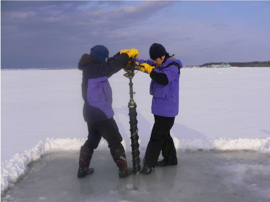
Ice sampling work. Investigations of the structure of lake ice is based on ice samples. The ice stratigraphy and crystal structure is studied in a cold room from the samples and ice impurities are taken from the meltwater.
