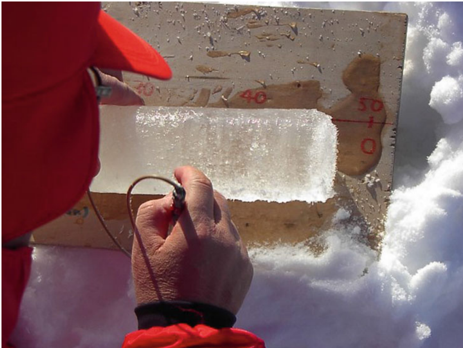
Fig. 3.4 An ice sample has been taken and, the visible structure is recorded and temperature profile is measured
