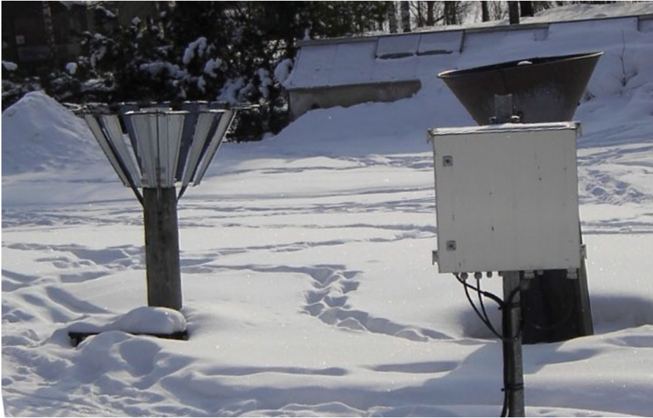
Fig. 2.9 Tretyakov model precipitation gauge with a snowfall capture system ( left side ). The metal slices around the cylinder constitute the specific design for aerodynamics to obtain good snowfall data. On the right, an old gauge behind the cabled box
