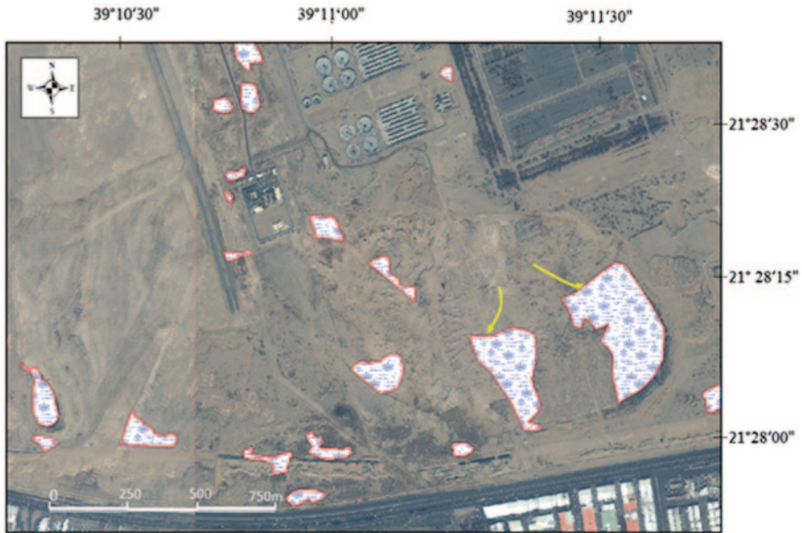
Fig. 9.23 Ikonos satellite image showing an example for locality No. 3 of the 3rd risk category. Water accumulated in depressions and low-lands
