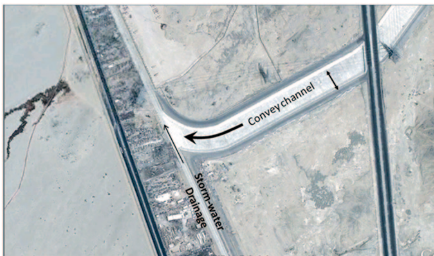
Fig. 10.11 Satellite image (Ikonos) showing the newly executed convey channel and the storm-water drainage with different dimensions at Wadi El Hatiel
