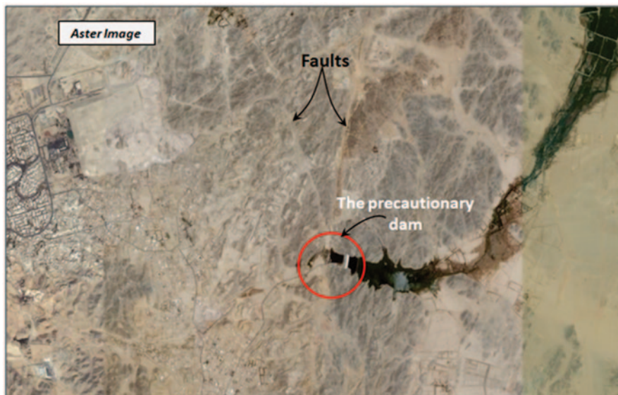
Fig. 10.12 The location of the Precautionary Dam at the intersection between two faults
