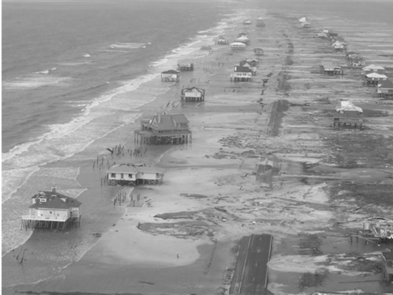
Fig. 14.7 The over-wash of Gulf of Mexico waters on Dauphin Island during hurricane Katrina in 2005
