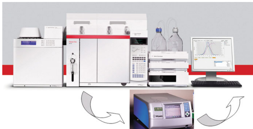
Fig. 3.1 HT-SEC system with built-in dual wavelength IR detector for concentration and chemical composition detection; system can be coupled to external MALLS detector (taken from [11] with permission of Polymer Char)
