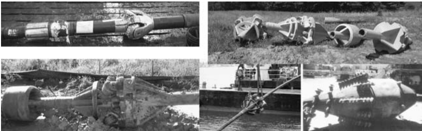
FIGURE 5.6 Different types of reamers. (Source: Trenchless Engineering Corporation.)
