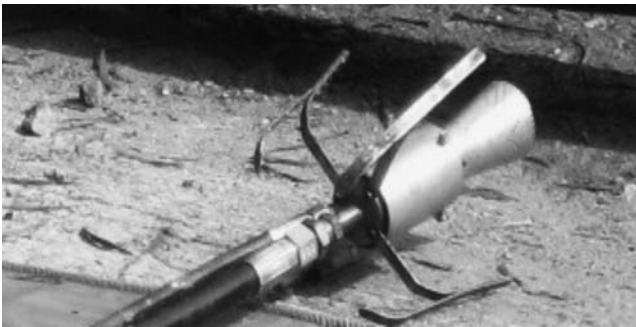
FIGURE 3.11 Polyurethane lining spray head. (Source: 3M Water Infrastructure.)
