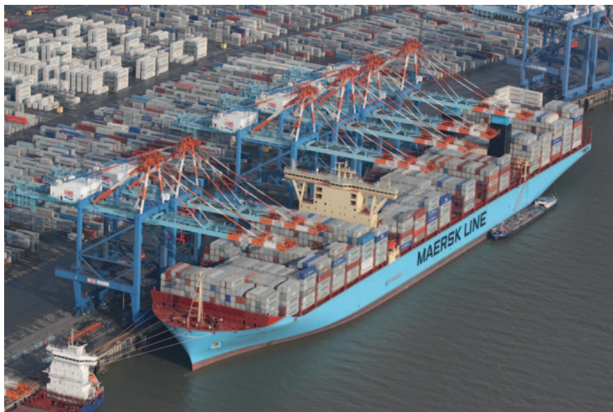
Fig. 2.37 A Mærsk Triple E class container ship (Mærsk Mc-Kinney Møller), one of the biggest ships in the world. An ice hockey rink, a football pitch, and a tennis court would fit on the deck simultaneously. Danish business conglomerate Maersk contracted Daewoo Shipbuilding to build 20 of these huge ships each of which can carry 18,000 containers. As of September 2014, eleven of the ships were ready. Some earlier supertankers were longer and heavier, but none of them are in service now. A highly energy efficient ship like this burns 100 t of Diesel a day. Cargo ships are responsible for about 4% of global air pollution. (Copyright-free Wikipedia picture)
