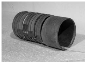
Figure 2: Equivalent of the tunnel lining with inner diameter of 76 mm created by hardened paper used in the model experiment.
