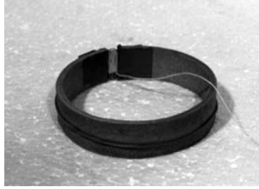
Figure 3: One ring used for the tunnel lining forming.
