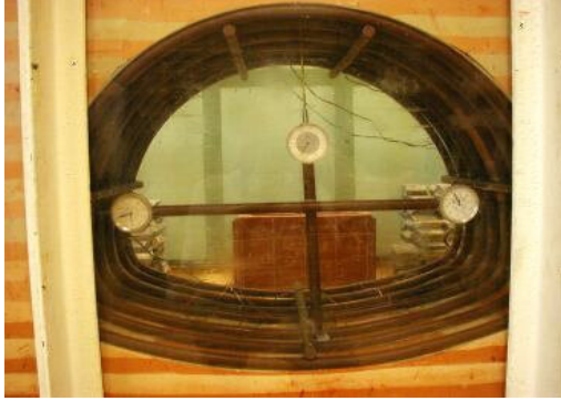
Figure 5: Detail of the tunnel with reinforcement and measuring equipments.
