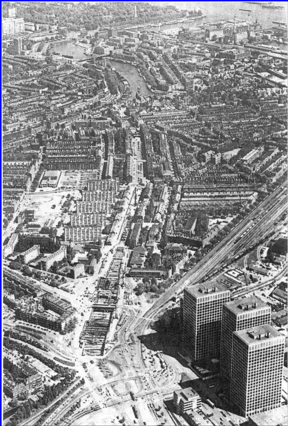
Figure 7. Tunnel trench through the heart of Rotterdam.
