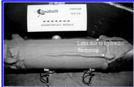
Figure 7. Model with bentonite after the test.
