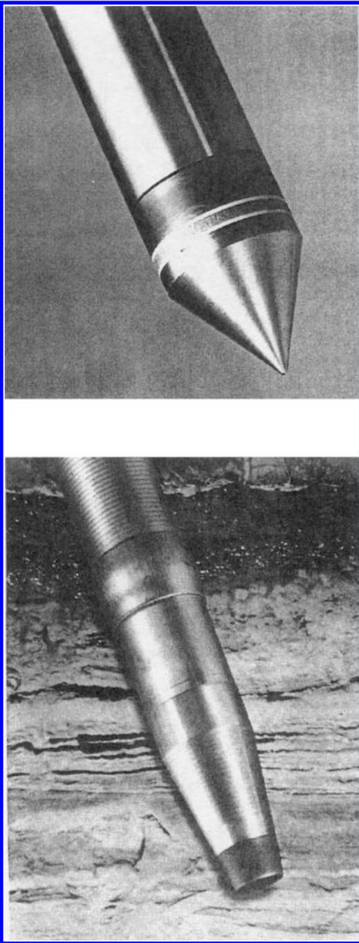
Figure 3. The CPT probe and the continuous sampler.
