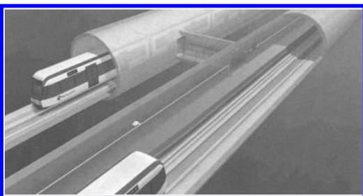
Figure 1. Two single track tunnels of 6.5 m diameter.
