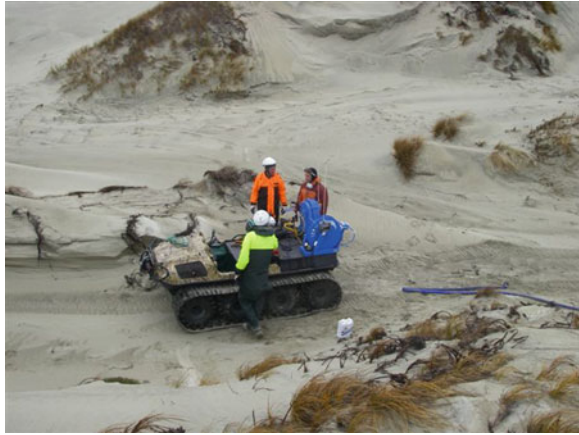
Fig. 5.13 Department of Conservation rangers spraying marram grass using an ARGO all-terrain vehicle equipped with a 500 liter spray tank and two 50 m hoses
