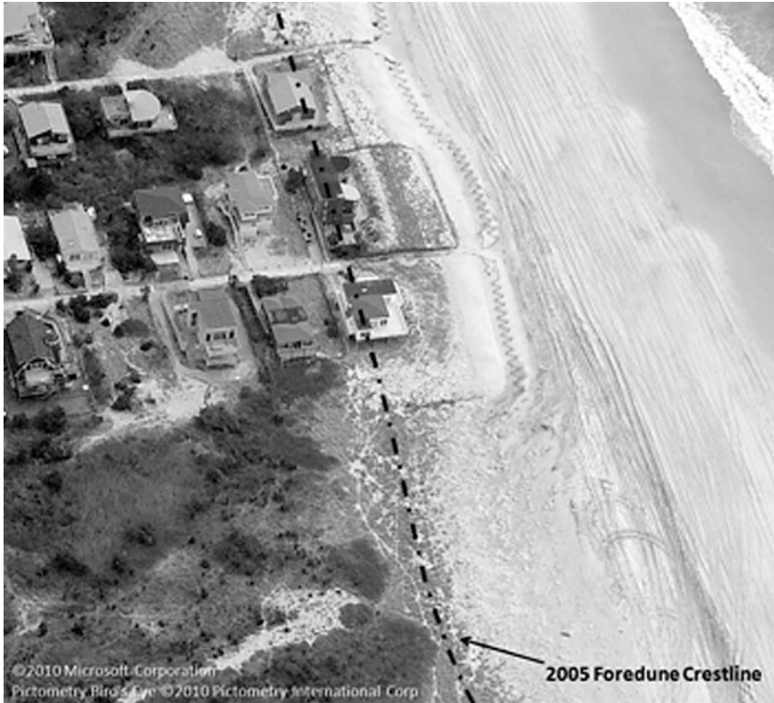
Fig. 3.10 Natural foredune crestline extending under or near the seaward margin of houses at Kismet. The constructed foredune is wiped out at intervals. The newly constructed foredune line has been sited farther seaward at the second house
