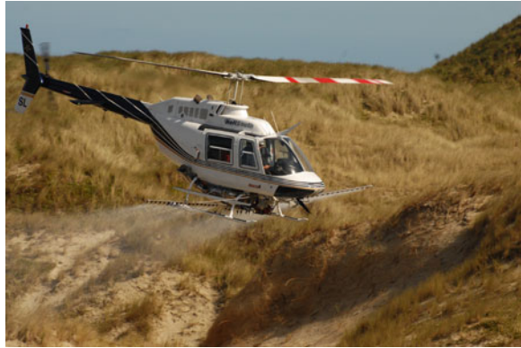
Fig. 5.12 A Jet-Ranger helicopter equipped with a spray boom, engaged in marram control operations, Mason Bay, December 2010
