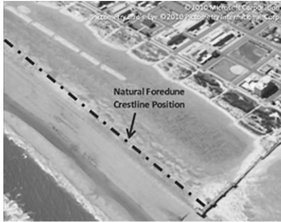
Fig. 3.11 The constructed foredune is maintained inland of its optimal position, Wildwood, NJ, USA
