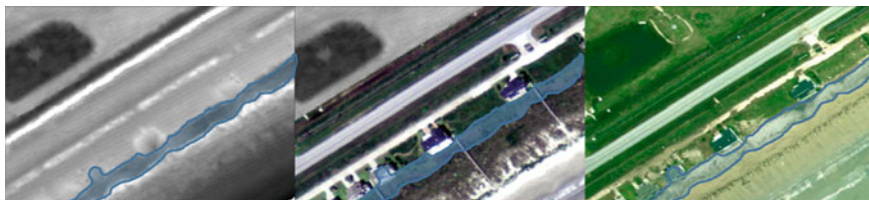
Fig. 6.3 Using a GIS–LIDAR–GPS survey approach to restoration. Hurricane Ike altered the dune and swale topography at the Sandhill Shores site. Left image shows pre-storm LIDAR elevation data, clearly indicating the swale and dune locations ( black is low elevation, white is high). Center image is pre-storm aerial imagery, right image is the post-storm image. In all three geo-referenced images, the outlined blue area denotes the same swale location, for comparison. Imagery courtesy of the TNRRIS
