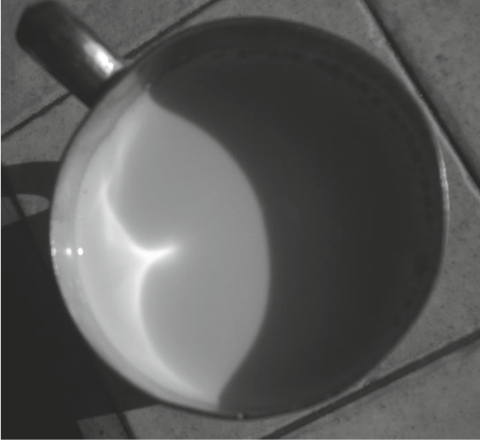
FIGURE IV.4 Caustics produce by reflection from the inner rim of a metal tankard. The shape produced in this common example is called a nephroid cusp (Copyright © C. R. Kitchin 2010).
