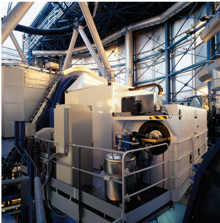
FIGURE 4.5 A modern general-purpose astronomical spectrograph (FLAMES – Fibre Large Area Multi-Element Spectrograph) for ESO's VLT. The spectrograph is the collection of room-sized boxes in the foreground. The 8.2-m Kueyen telescope is in the background and gives an idea of scale. (Reproduced by kind permission of ESO/H.H.Heyer).
