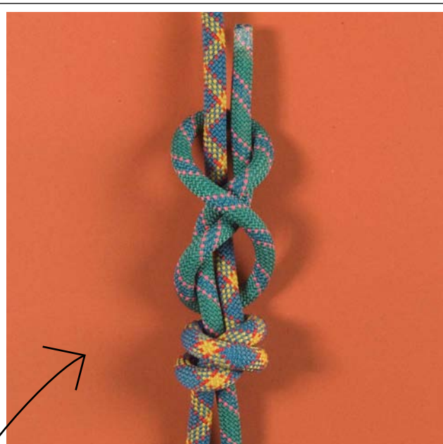
Double Fisherman's Knot: Step 4
