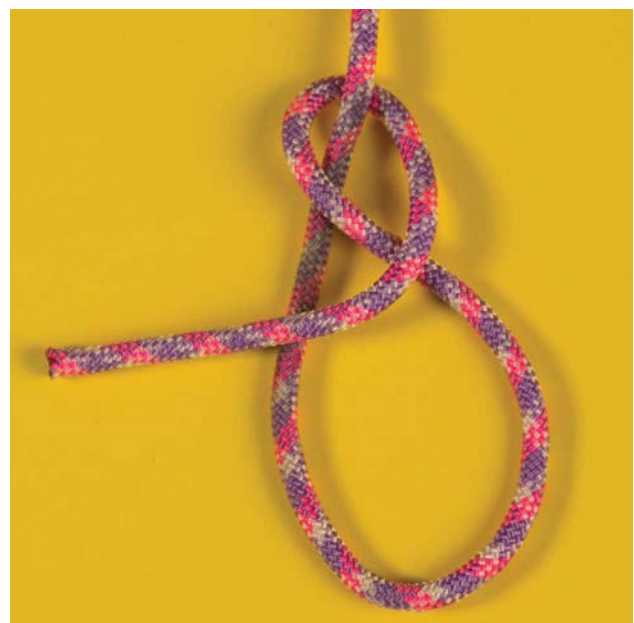
Scaffold Knot: Step 2
