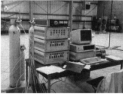
Figure 8: Constant concentration tracer gas equipment using N 2 O as a tracer gas.
