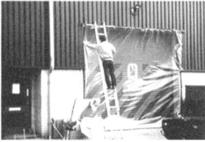
Fig 2: The 'leaky' roller shutter door of a small factory unit is being sealed to assess its contribution to the overall air leakage.
