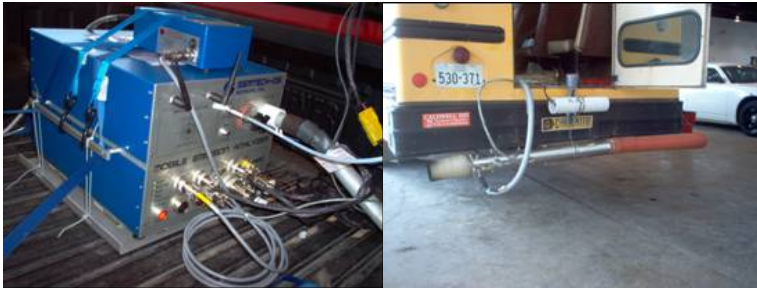
Figure 1. Components of the SEMTECH-DS unit installed on a school bus.
