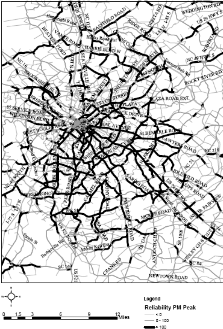
Figure 2. Reliability in terms percent variation in travel time during evening peak period.
