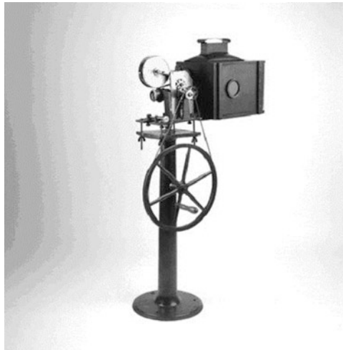
Fig. 7.3 Robert Paul's Theatrograph projector. The handle on the large wheel is for winding the film through. The big black box at the rear is the lamp house. It isn't clear which type of light is being used. Source: http://cinemathequefrancaise.com/Chapter3-1/Figure_03_06_Theatrograph.html
