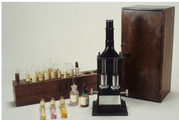
Fig. 6.7 Bausch and Lomb Duboscq type colorimeter. Photo by Gregory Tobias. Courtesy of the Chemical Heritage Foundation Collections
