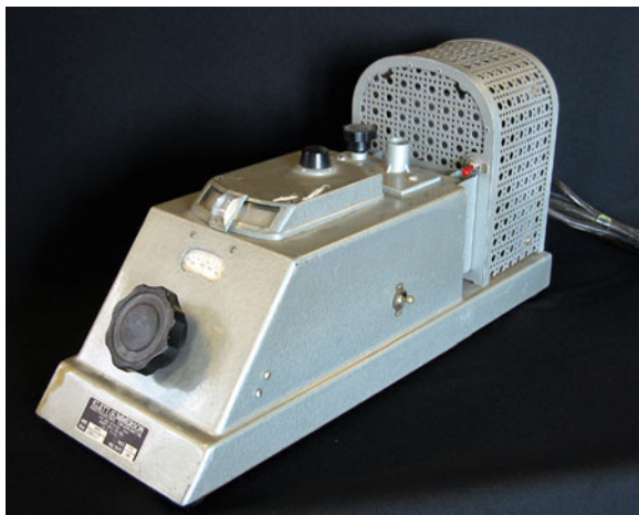
Fig. 6.8 Klett-Summerson photoelectric colorimeter, clinical model. Photo by Gregory Tobias. Courtesy of the Chemical Heritage Foundation Collections
