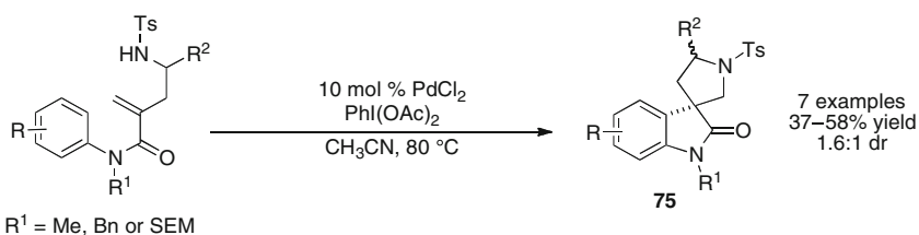
Scheme 56 Synthesis of spirooxindoles via intramolecular alkene aminoarylation
