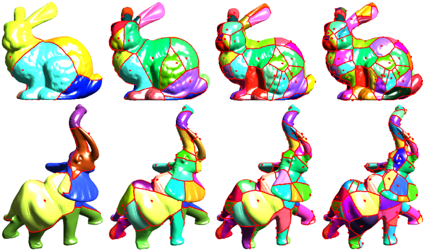
Fig. 2.21 Example of Voronoi segmentations for an increasing number of seeding points
