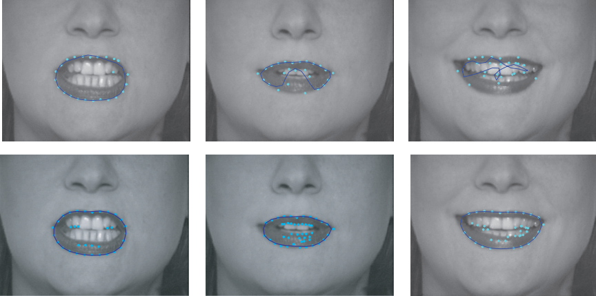
Fig. 3.11 Tracking results with Kalman snakes (top row) and S-PDAF (bottom row) (From [16], 2004 IEEE)
