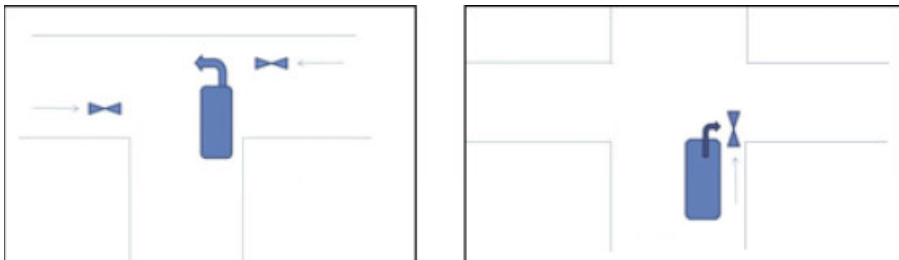
Figure 16.2. Critical cyclist scenarios: a) vehicle pulling out into the path of an oncoming cyclist at an intersection; b) vehicle turning into the cyclist's path
