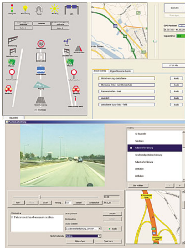
Figure 15.1. Screenshot of graphical user interface of Eves, a) during inspection b) and post-processing [NAS 11]
