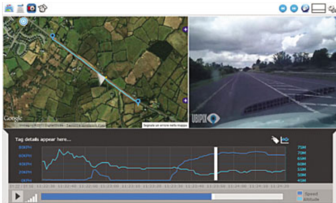
Figure 15.3. Road Safety Inspection in Ireland using UBIPIX
