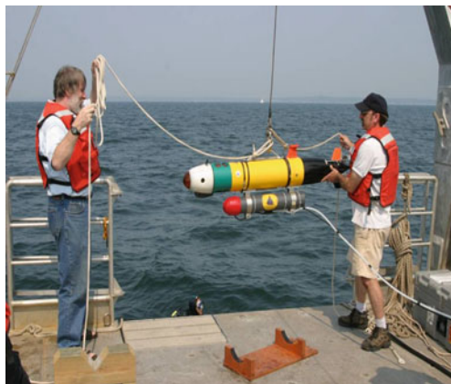
Fig. 8.13 Deployment of REMUS AUV carrying a towed acoustic array in shallow water off Nantucket Sound, MA
